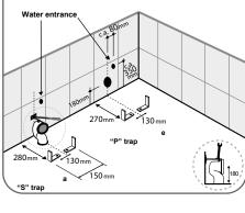
2 - Install flushing mechanism in the cistern. Prepare the connection for the cistern flushing according to the given dimensions. Place the WC concealing brachets and push it to the wall. We suggest lubricating both sides to make the connection easier, ensure alignment of both pieces.
