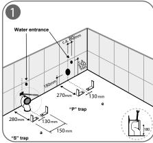
1 - Prepare the water inlet, the soil pipe connection and the fixing screws according to the given measurements depending on your trap type
