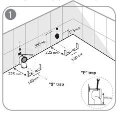
1 - Prepare the drainage and fixing screws according to the given measurements depending on your trap type
