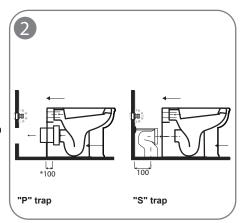
2 - Prepare the connection for the cistern waste. Assemble the drainage connection on the WC, then place the WC on the fixing brackets and push against the wall
