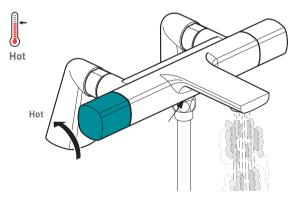
Turning the temperature control handle in the direction of the arrow increases the water temperature
