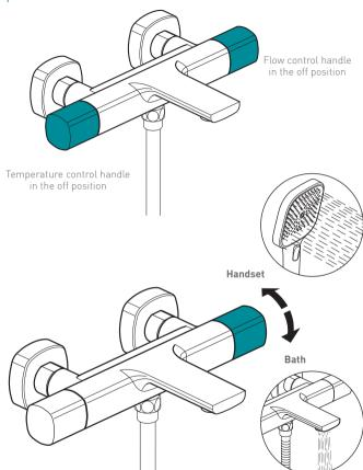
Turning the flow control handle in the direction of the arrows diverts the flow of water to the handset or bath
