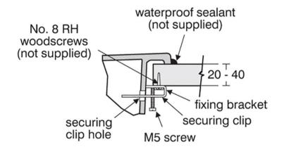
section through basin showing securing clip
