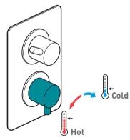
Turning the temperature control handle in the direction of the arrows increases/decreases the temperature
