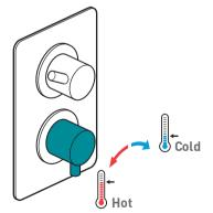
Turning the temperature control handle in the direction of the arrows increases/decreases the temperature
