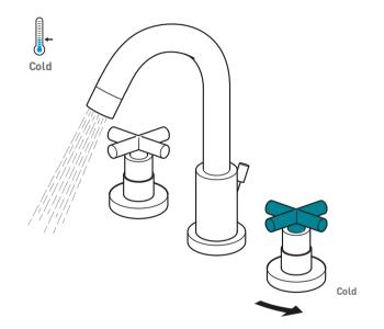
Turning the cold handle anti-clockwise will increase the flow of cold water.
