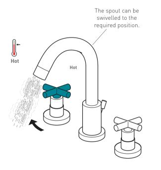
Turning the hot handle clockwise will increase the flow of hot water.
