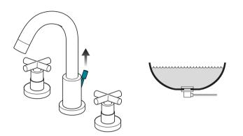
Pull the waste control rod up to close the plug and fill the basin.
