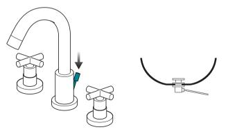
Push the waste control rod down to open the plug and empty the basin.
