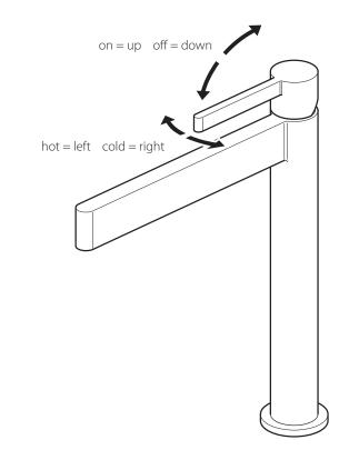
Moving the mixer lever upwards/downwards will increase/decrease the flow of water. Moving the mixer lever from right to left will increase the water temperature.
