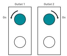
Turning the flow control handle in the direction of the arrow increases the flow of water to the outlet.
