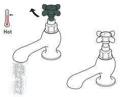
Turning the hot handle clockwise will increase the flow of hot water.
