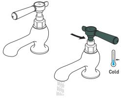
Turning the cold handle anti-clockwise will increase the flow of cold water.
