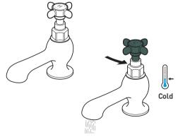
Turning the cold handle anti-clockwise will increase the flow of cold water.
