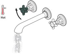
Turning the hot handle clockwise will increase the flow of hot water.
