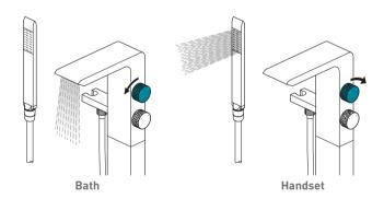
Turning the diverter handle anti-clockwise activates the flow of water progressively to the bath Turning the diverter handle clockwise activates the flow of water progressively to the handset
