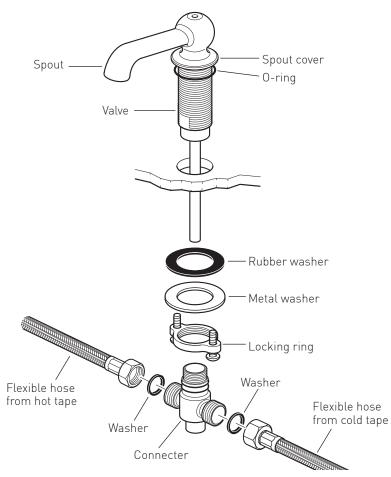
Make sure the O-ring is in place in the underside of the spout cover.
