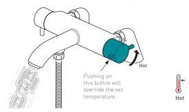
Turning the temperature control handle in the direction of the arrow increases the water temperature
