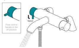
Turning the flow control handle in the direction of the arrow increases the flow of water to the spout
