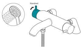
Turning the flow control handle in the direction of the arrow increases the flow of water to the handset
